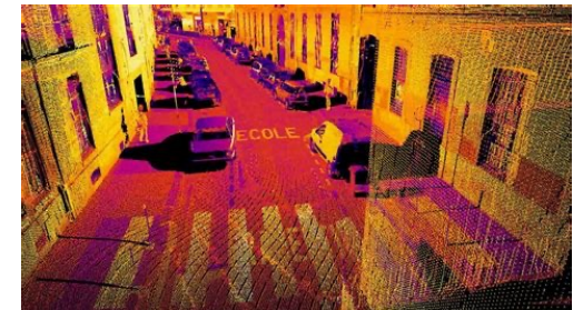
3D point cloud color with backscatter intensity
